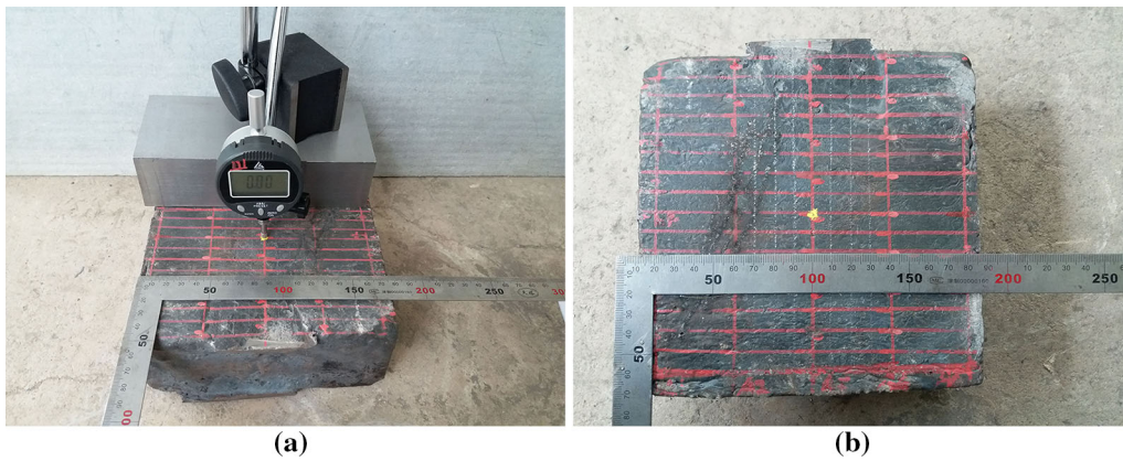
Fig. 4—Roughness measurements (a) measuring device, and (b) grid of measured points on ingot surface.
