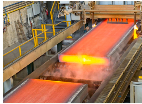
(b) Cutting a slab from the strand exiting a continuous-caster (Primetals Technologies, 2019)
